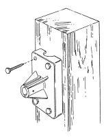
3. Drive the lag screws through the holes in the anemometer base and into the wood.
