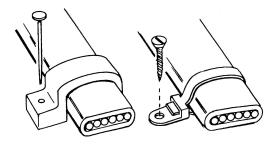
Note: Do not use metal staples to secure cables. Metal staples can cut the cables.
