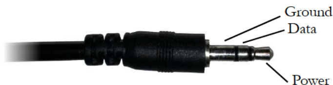
Figure 5: 3.5 mm Stereo Plug Wiring
