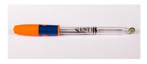
Glass combination pH electrode for use in drinking water, low ionic strength or low temp. sample applications, Double-junction, sealed, ceramic junction, Ag/AgCl reference
