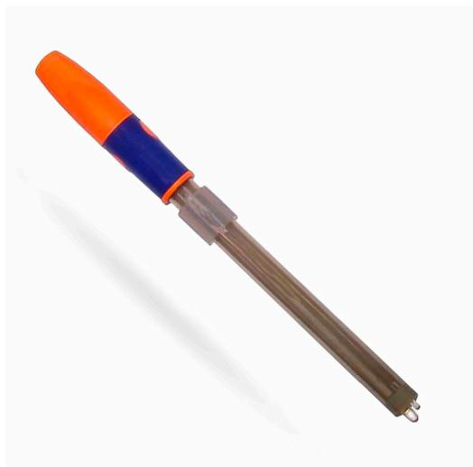
Jam pH Electrode, Body Type: Epoxy, Junction Type: Replaceable Ceramic, Connector: BNC, Easy penetration, cleaning and maintenance, Dimensions: 120x12mm, Wet Material: Glass, Ceramic, Ref. Type: Single Junction Ag/AgCl
