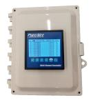
8 Channel Programmable Controller for O2 or Gas Monitors
