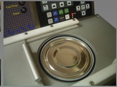
Can loaded, top down. Closing Lid will start test.
