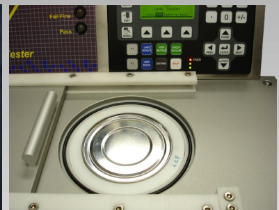
Small can loaded, within annular insert.
