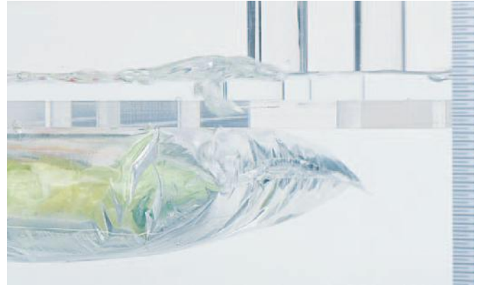
The Pack-Vac’s clear tank provides 360° viewing. A telltale stream of bubbles will rise from a leak.
