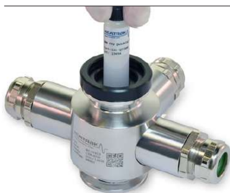
QuickCal “liquid free” ISO 7027 formazine turbidity calibration.
