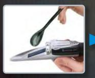
1 Apply 1-2 drops onto the prism.
