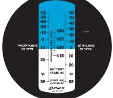
For measuring concentration of antifreeze solution for automobile radiator at gas station, service station, etc.
