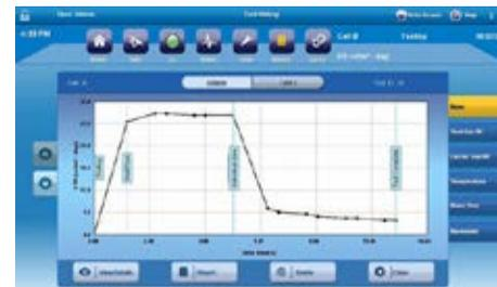
*Sequential testing allows a series of tests to be performed on the same samples at different test conditions*
