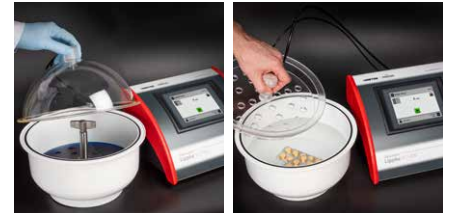
Methylene blue dye test with domed lid
